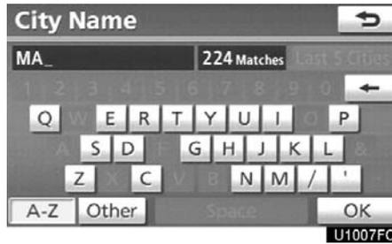
To search for an address or a name, touch “OK”. Matching items from the database are listed even if the entered address or name is incomplete.
