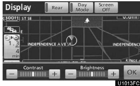
**To display the screen in day mode even with the headlight switch on, touch “Day Mode” on the adjustment screen for brightness and contrast control.**
